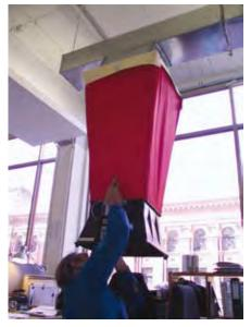
Checking air flow readings from supply air diffuser (Source: AIRAH)
