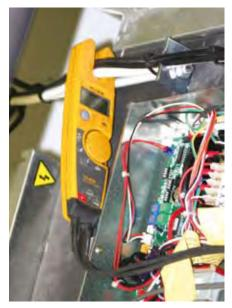
Typical clamp meter used by HVAC technician to check correct electrical current (AIRAH)
