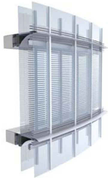
1 3D View Detail - Double Skin Facade (Blinds Down)
