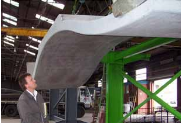
Figure 19 – CH2 precast panel
