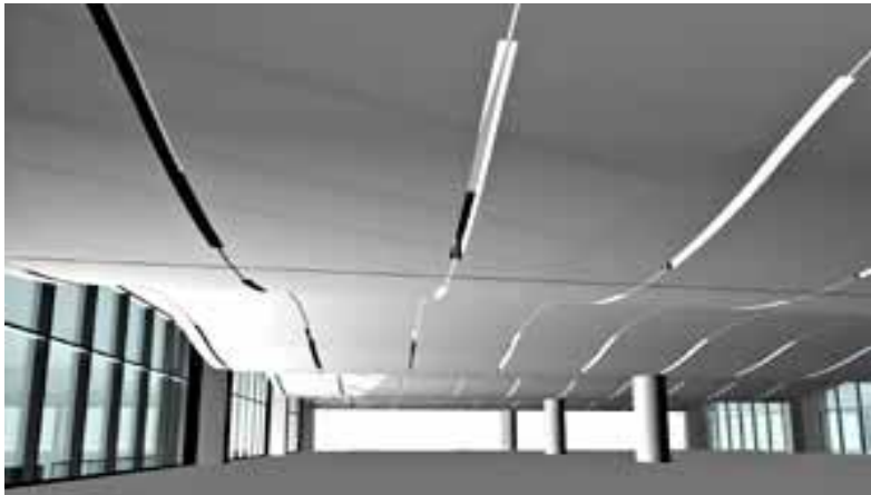
Figure 28 - computer model of the office spaces with precast concrete ceiling-floor system (DesignInc)
